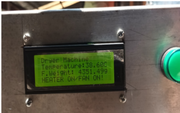
Figure 8. LCD reading of the Automated Dryer
