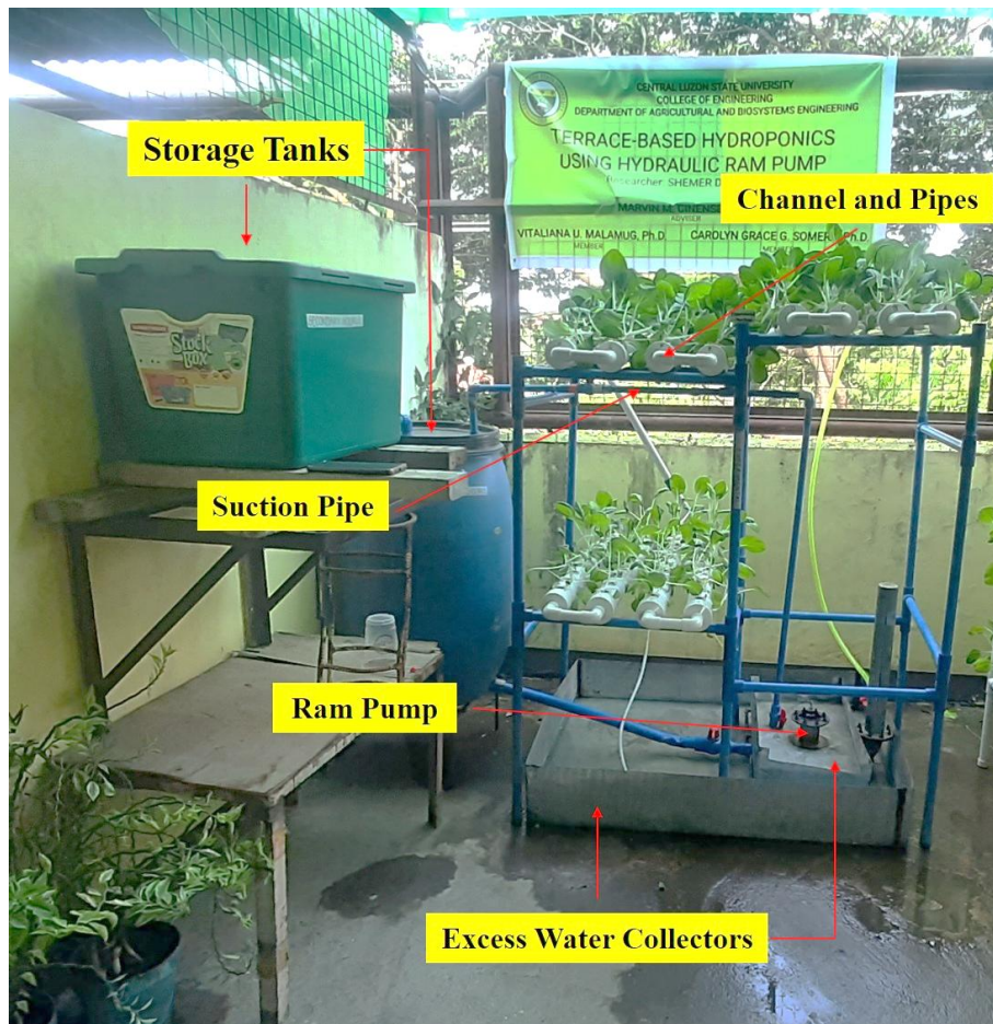
Figure 3. Fabricated terrace-based hydroponics system using hydraulic ram pump
